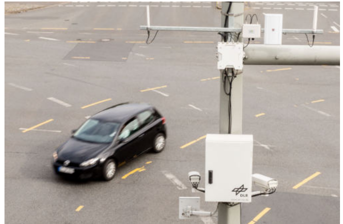
Fig. 1. Example of a camera system operated by DLR. Detail of a camera mast in Braunschweig at the research intersection. The installations carry further hardware for e.g. communication.
