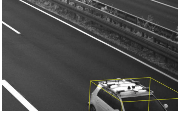
Fig. 4. Correct estimation of the bounding box around a car only partially visible in the scene.
