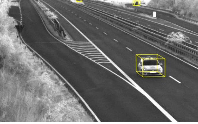
Fig. 2. An example perspective recorded at Test Bed Lower Saxony. An RTK-corrected reference trajectory recorded by the car moving towards the camera is used for the evaluation in this article.
